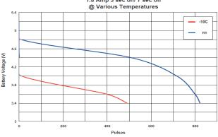
Delivered capacity is dependent on the applied load, operating temperature and cut-off voltage. Please refer to the charts and discharge data shown for examples of the energy/service life that the battery will provide for various load conditions.
